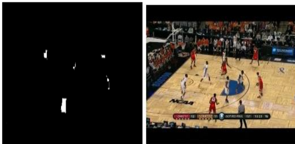
Figure III. The binary thresholded image after a morphological close operation: The original first frame of the sample video (left) and the final binary court mask of the first frame (right)
