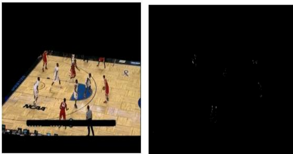
Figure II. A video frame multiplied by the binary court mask(left) and The binary court masked video frame after being threshold based on Ohio St.'s trained YCbCr values(right)
