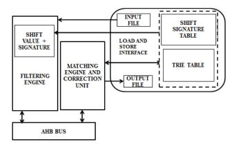
**Figure I.** Virus Detection/Correction Processor Architecture
