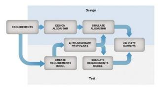
Figure II. Model-Based Testing Processor
