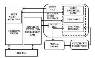
**Figure III.** Virus detection and Testing Processor architecture
