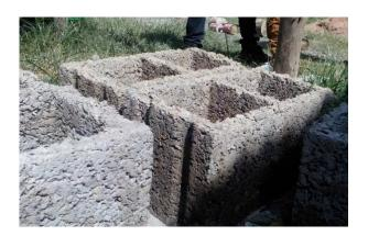
Figure II Prepared sample hollow blocks
