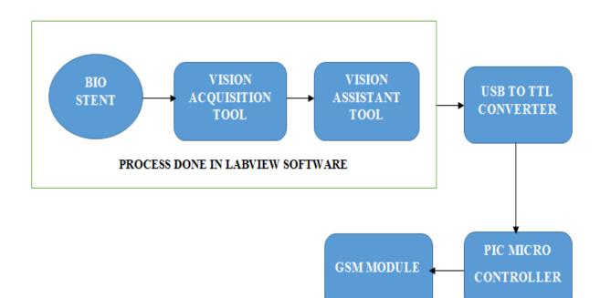
Biodegradable stent images are analyzed and compared in LABVIEW software. Image display- This control is used to create Region of Interest (ROI). Classic and 3D images are available in this control panel. Machine vision-
