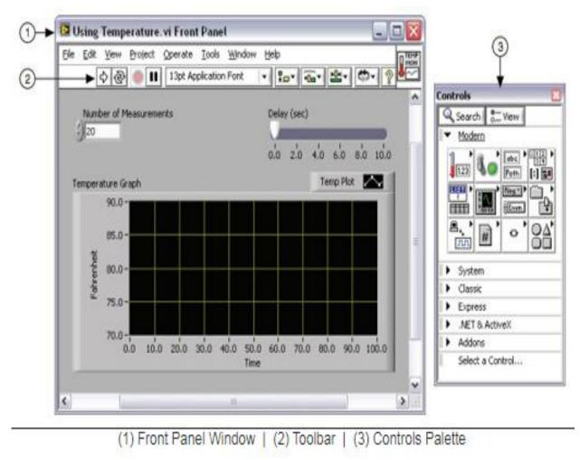
Figure I. Front Panel of LABVIEW
