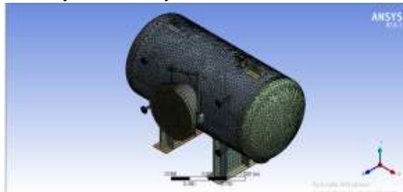
Fig 2: Fine Mesh generated in ANSYS
