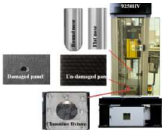
Figure 2: Schematic of INSTRON™ 9250HV tester
