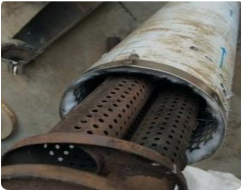
Fig 1: Faults in Automotive Muffler
