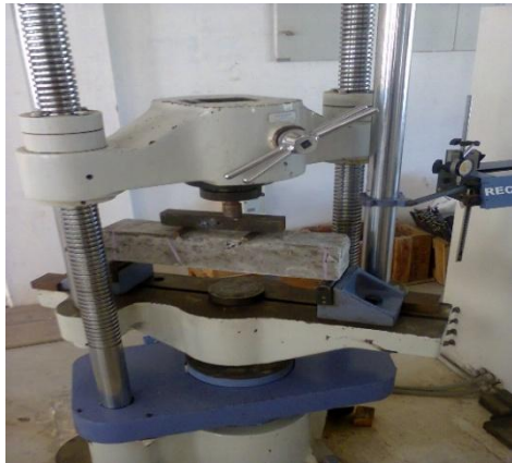
Figure 5. Instrumentation of beam specimen for flexural strength test
