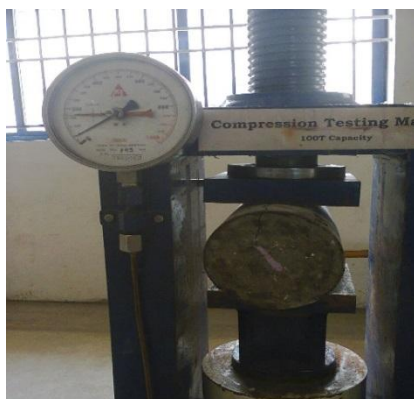
Figure 3. Instrumentation of beam specimen for Tensile strength test
