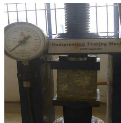
Figure 1. Instrumentation of beam specimen for Compressive strength test
