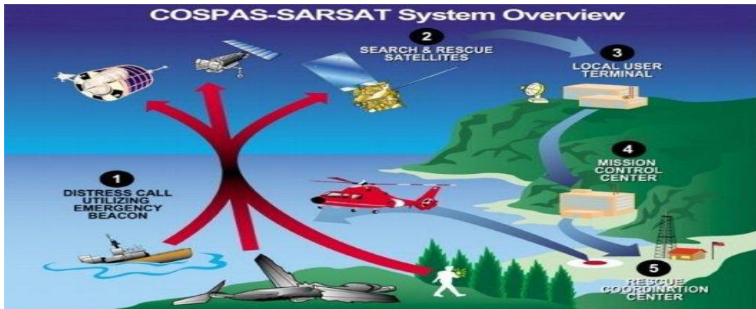
Figure 16. COSPAS-SARSAT System Overview
