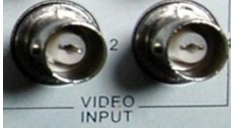
2. Bayonet Neill–Concelman, BNC Video Input
