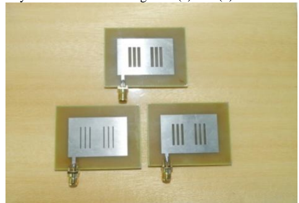
Figure 6. Antenna with variation in Slot width S_W = 0.5 mm, 1 mm and 1.5 mm.
