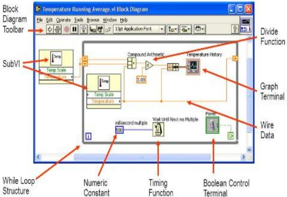
Figure II. Temperature Running Block Diagram
